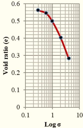
**Figure 4.** Pressure-void ratio curve for parent soil
