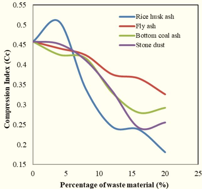
Figure 5. Variation of compression index for various soilsamples
