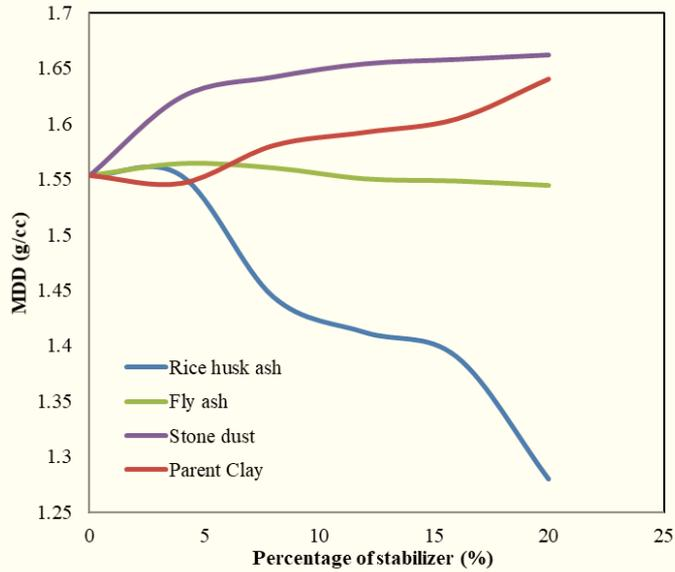
**Figure 2.** Maximum dry density for various soil samples
