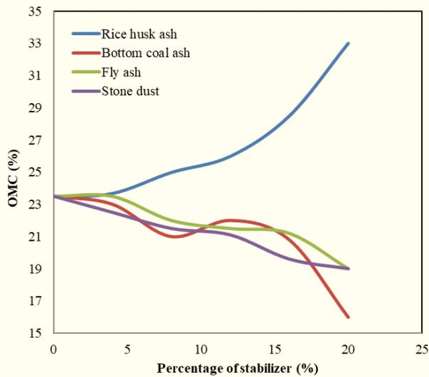
**Figure 3.** Optimum moisture content for various soilsamples
