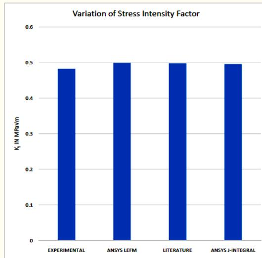
The obtained result was also verified using the J-integral approach. It was further verified using the analytical formula for a plate with a side crack under tension [32]. It can be observed that all the results are very close and the error involved is minimum.
