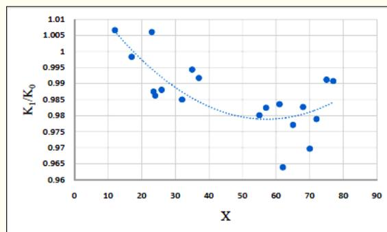
Since due to drilling of the hole effective cross sectional area decreases at the crack tip SIF increases. It was seen that for the present geometry considered the hole at a distance of 62 mm beyond which the effect of presence of hole becomes insignificant. Now keeping this lateral distance as constant perpendicular distance is varied and its optimum position is identified.
