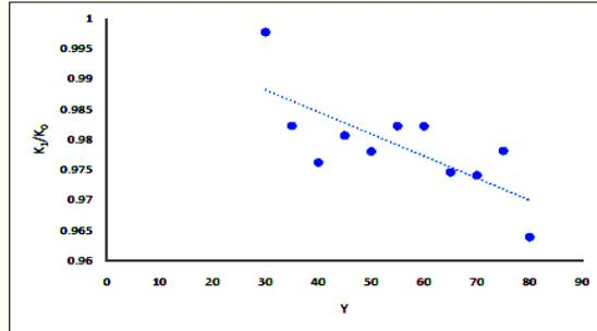
Presence of stop hole very near results in decrease of SIF however it decreases with further movement of the stop hole. However after a certain position its effect becomes insignificant and the SIF starts increasing ultimately reaching the previous value of SIF (plate without hole).
