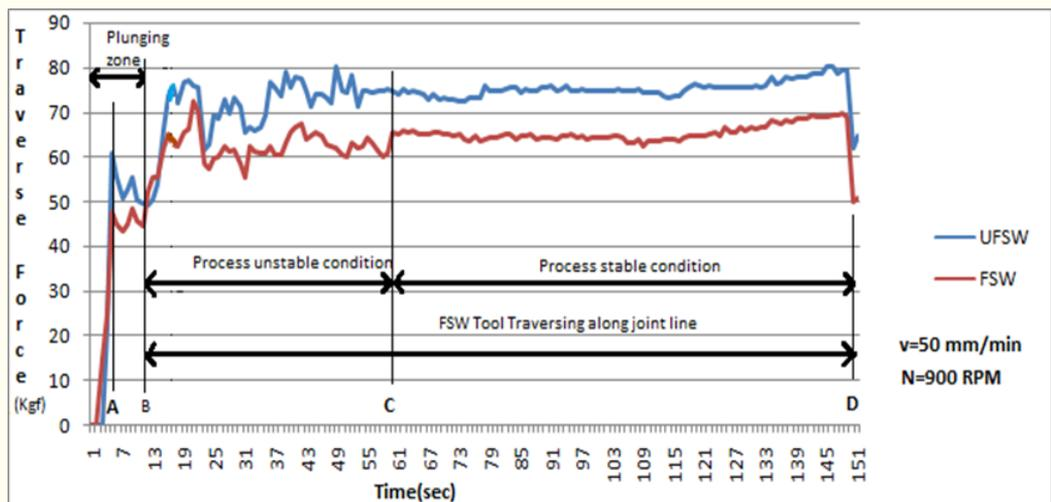
Figure 6. Traverse force applied by FSW tool
