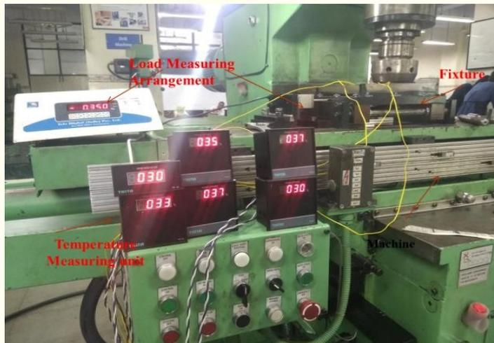
Figure 2. FSW arrangement with temperature and load cell measuring unit
