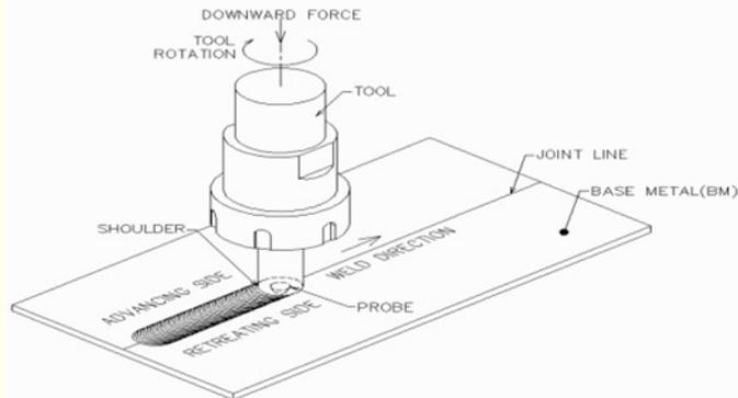
Fig.1. Schematic representation of FSW [6]
