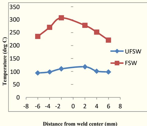
Figure 5. Distribution of temperature at AS and RS for different cooling media
